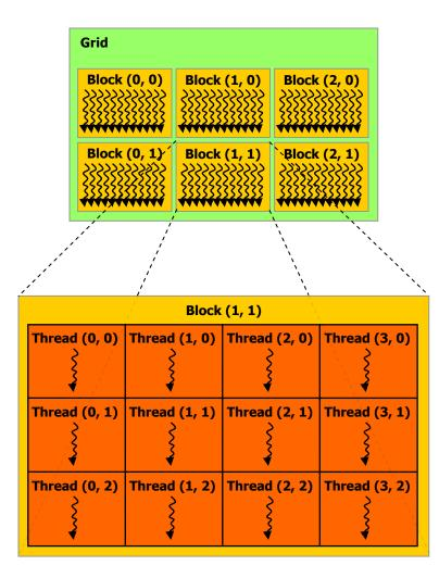
Figure 2-1. Grid of Thread Blocks
